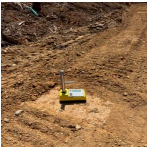
Performing density tests using Troxler Nuclear gauge
