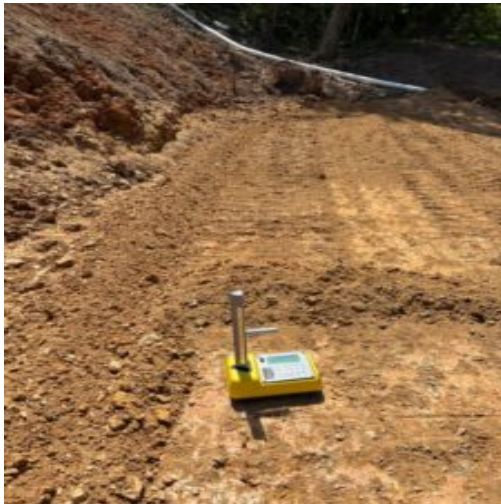
Performing density tests using Troxler Nuclear gauge
