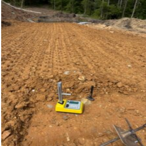
Performing density tests using Troxler Nuclear gauge
