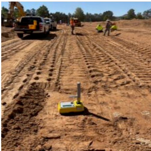
Density tests performed on sanitary sewer line backfill between structures Z15 and Z16
