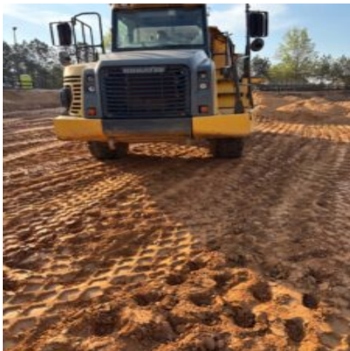
Proof roll indicating moderate to severe movement
