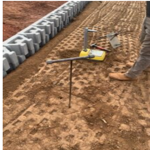
Performing density tests probing and using nuclear gauge
