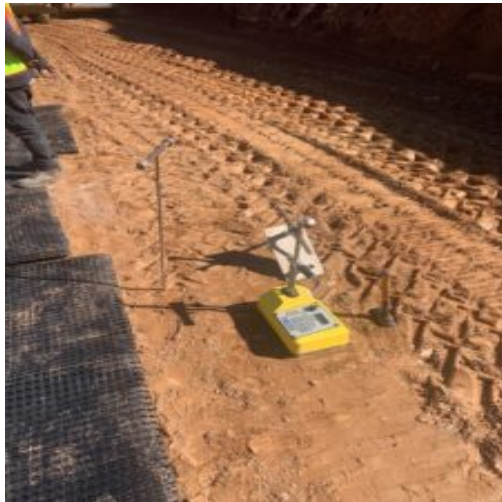
Performing density test using Nuclear gauge
