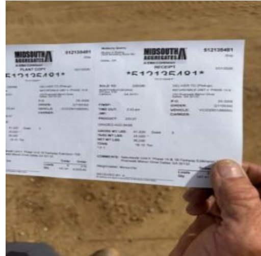
Ticket showing 18.10 tons of base stone
