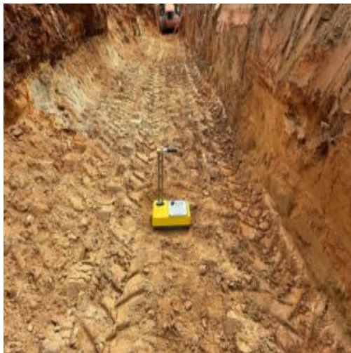
Field density test between manhole 9 and 8
