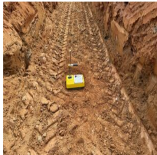
Field density test between manhole 9 and 8
