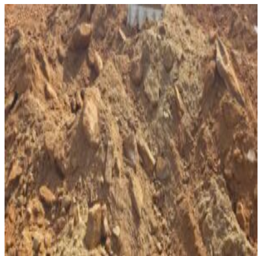
backfill material mixed with finer soil
