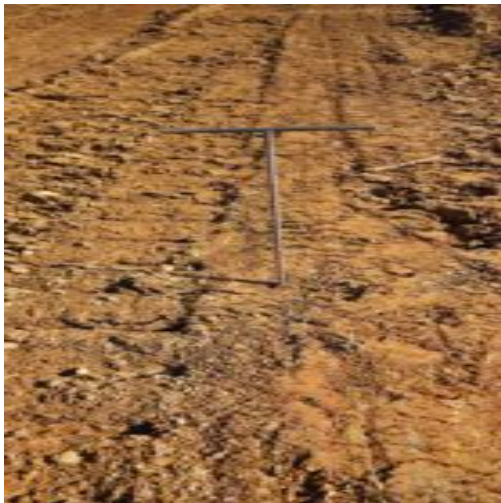
pumping/failed probe rod (addressed by contractor)
