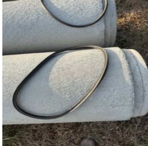
Rubber seals and 18 inch storm drain
