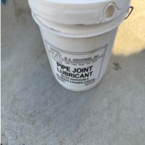
Lubricant for 18 inch storm drain
